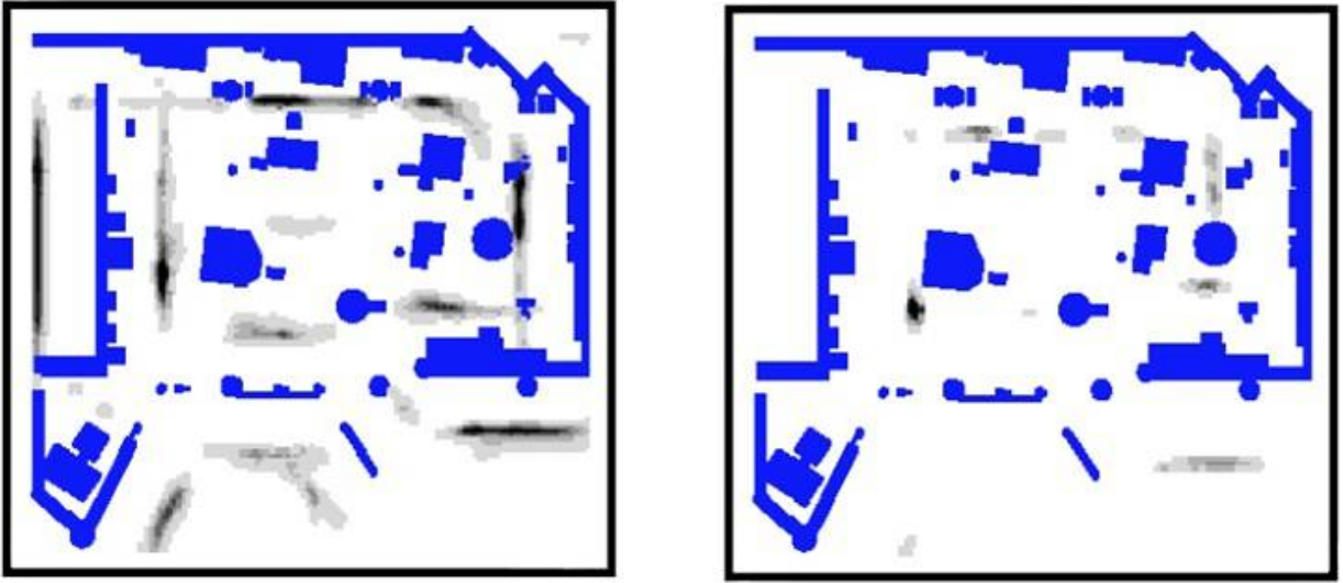
Figure 12: Left map shows possible places on the map where the robot could be. The right map shows the situation after a few minutes. The search area is now more focused around the actual position of the robot.
